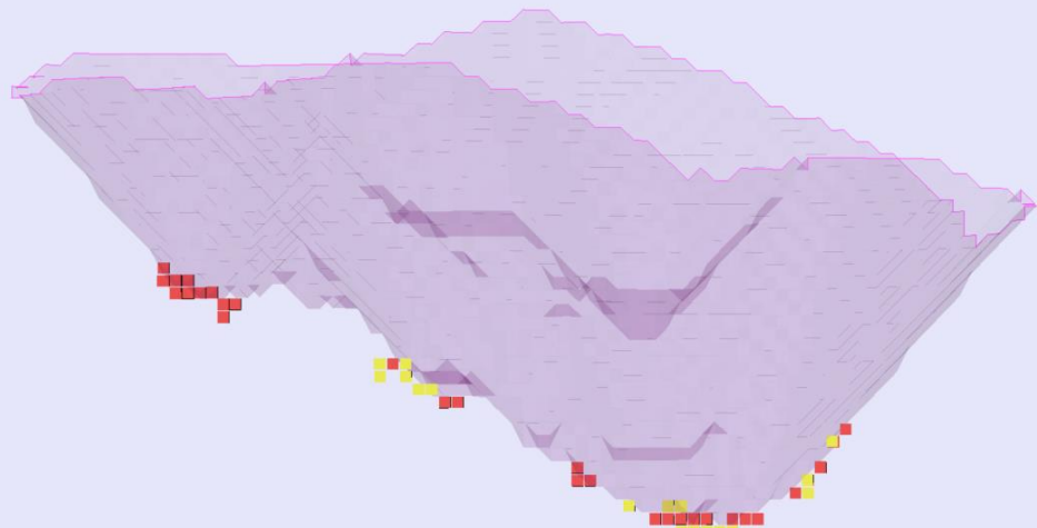
Long section showing El Rubi pit shell with underground blocks >1.4g/t gold OR 106 g/t silver
